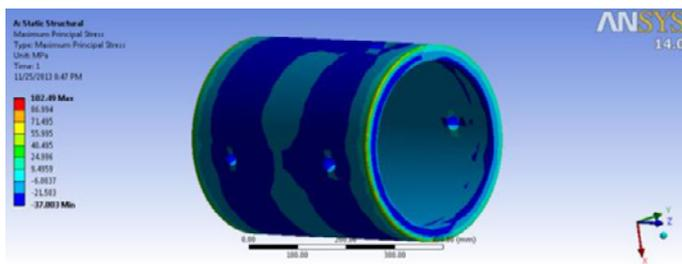
**Figure 2.** Maximum principal stresses on the main body of the chamber.
