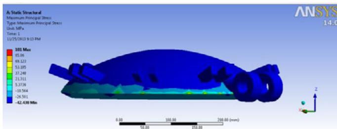
**Figure 3.** Maximum principal stresses the ellipsoidal top head of the chamber.
