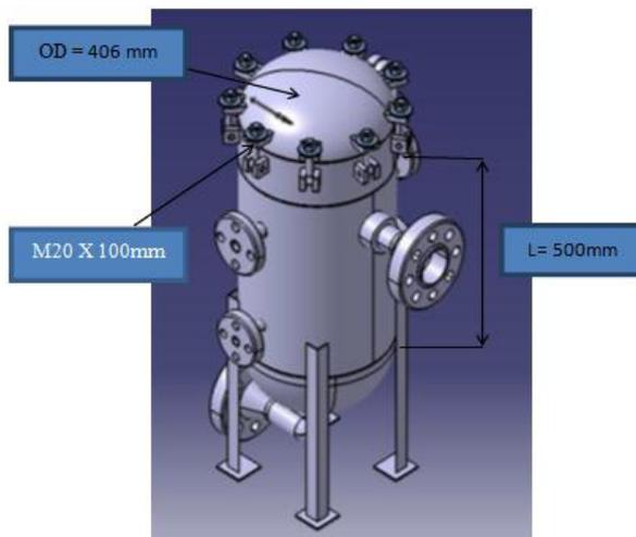
**Figure 1.** Isometric view of the hyperbaric chamber.
