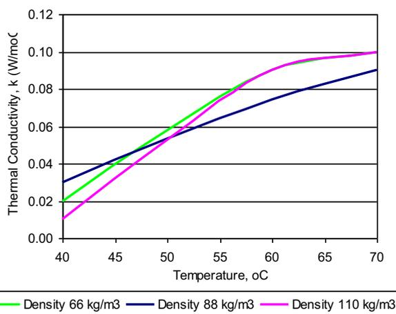
**Figure 1.** Thermal conductivity values for the different packing density
