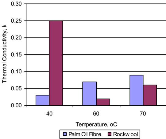
**Figure 2.** *k* values of palm oil fibre and rockwool at different temperatures
