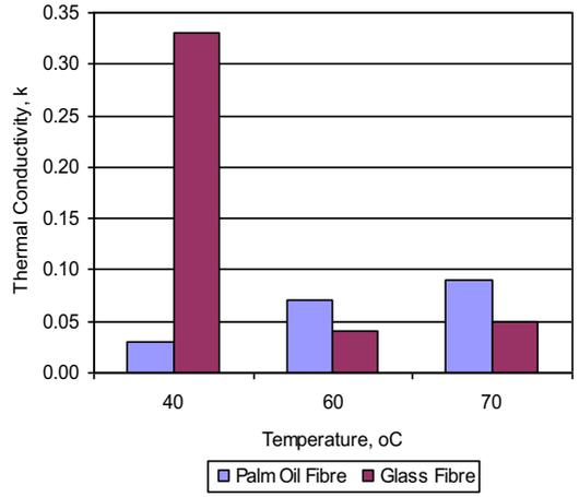
**Figure 3.** *k* values of palm oil fibre and glass fibre at different temperatures
