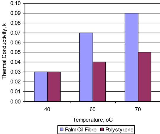
**Figure 4.** *k* values of palm oil fibre and polystyrene at different temperatures
