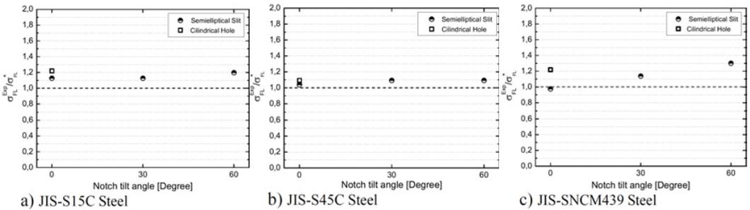
Figure 2. Fatigue limit as a function of the tilting angle of defect for three types of steel.
