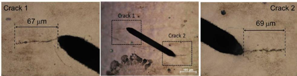
Figure 3. Non-propagating cracks found at the fatigue limit (JIS-SNCM439, Defect type B,  $\sigma_{FL}^{exp} = 260$  MPa).
