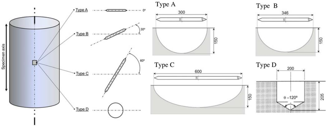
Figure 1. Geometries and orientations of artificial defects.
