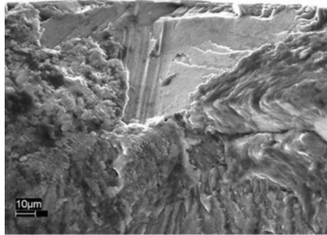
**Figure 2.** Crack initiated from as-forged surface.
