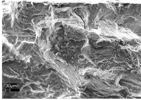
**Figure 3.** Crack initiated from machined surface.
