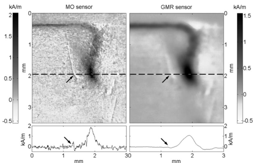
**Figure 1.** a) MO measurement of the middle section of specimen-4; b) multi-line GMR measurement of the same location; underneath each plot: the distribution of the SMLF along the dashed line. Arrows mark the location of the SNR evaluation. (Images were enhanced for publication purposes.)
