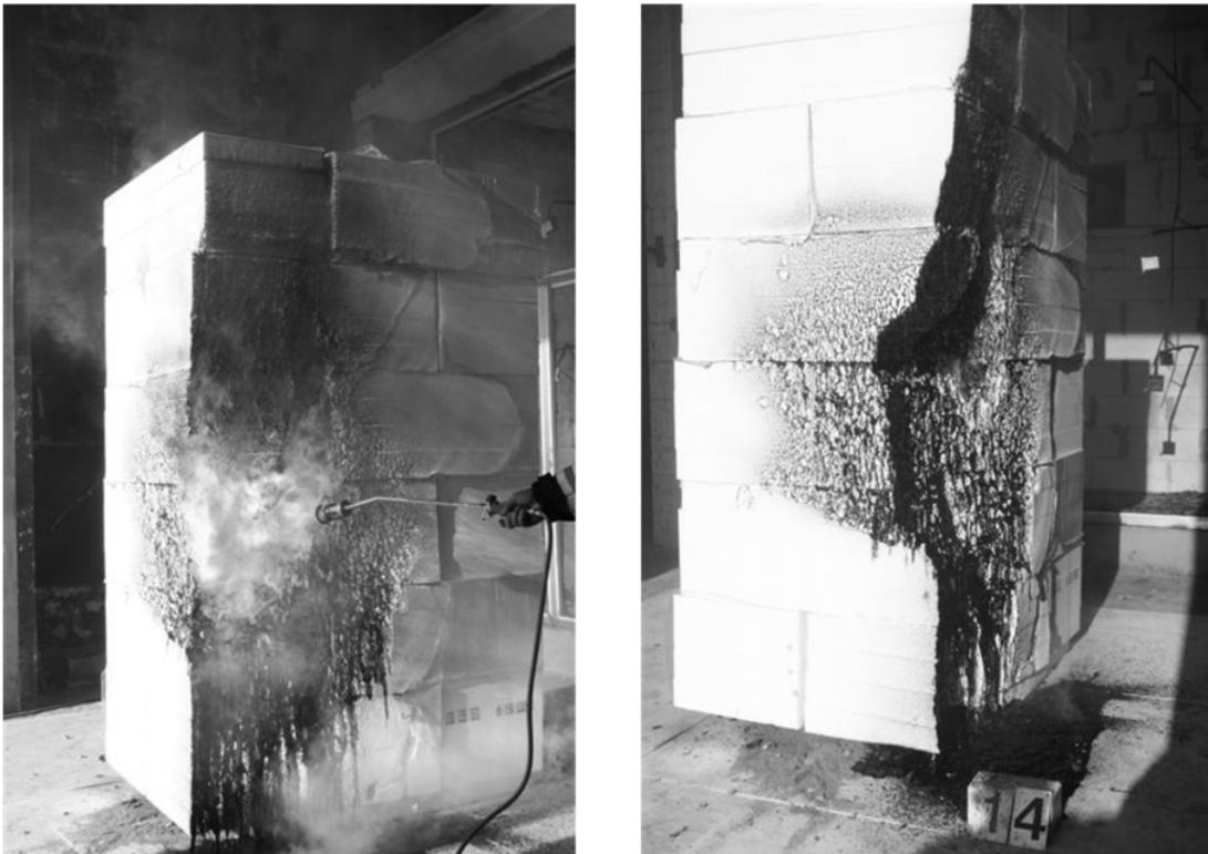
**Figure 1.** Flame retarded (class E) EPS during and after flame impingement with gas burner.
