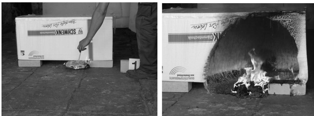
**Figure 2.** Paper cushion ignited below stored EPS – Melting but no continuous burning of EPS.
