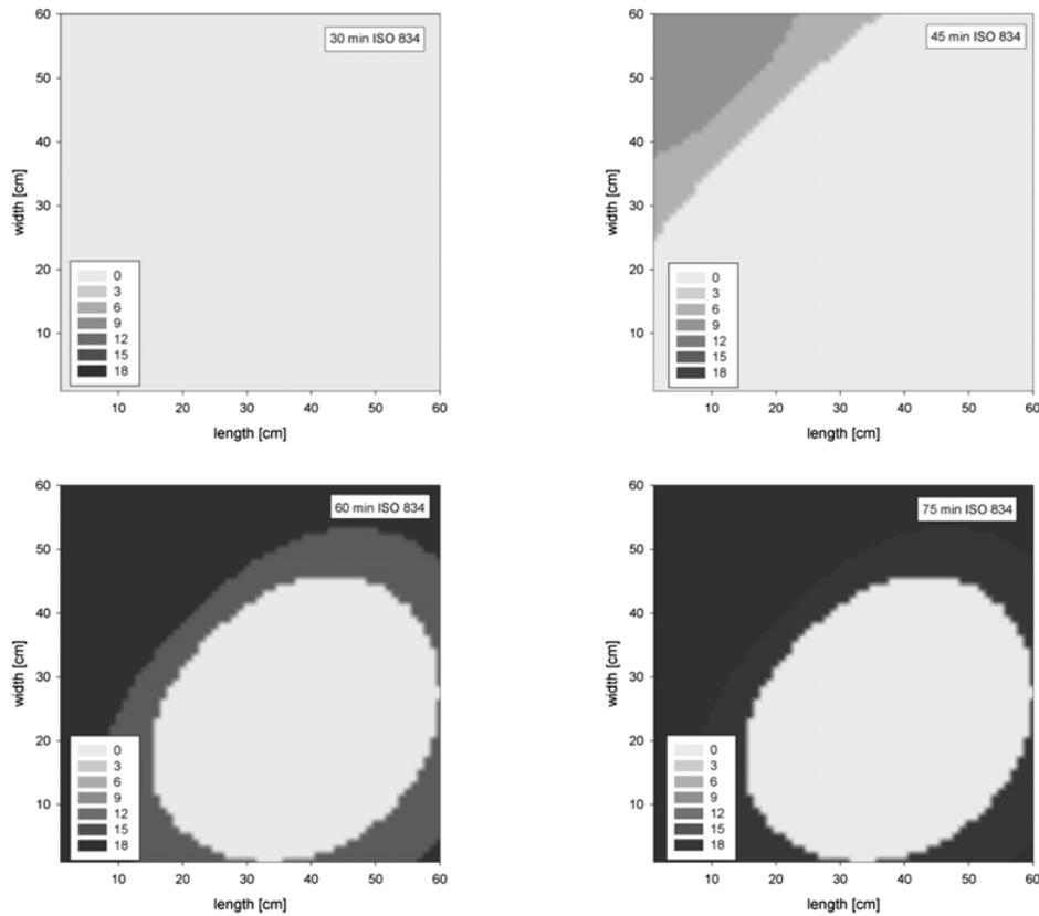
**Figure 3.** Example 1 of the spatial occurrence of spalling for a concrete slab with mean  $f_{ct,20^{\circ}C}$  of class 6 (3.1 MPa) for different ISO 834 durations – first realization of the random field.
