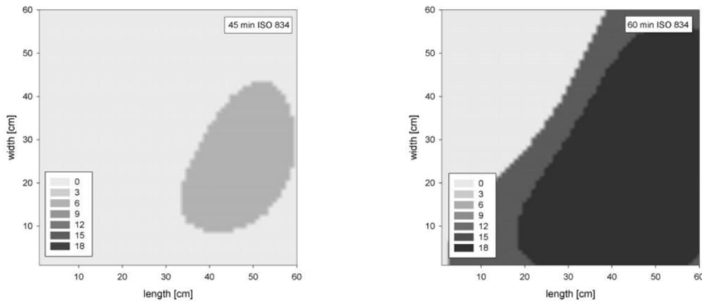
**Figure 4.** Example 2 of the spatial occurrence of spalling for a concrete slab with mean  $f_{ct,20^{\circ}\text{C}}$  of class 6 (3.1 MPa) for different ISO 834 durations – second realization of the random field.
