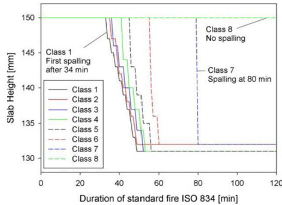
**Figure 2.** Spalling behavior for different classes of  $f_{ct,20^\circ C}$  as a function of the fire exposure time.
