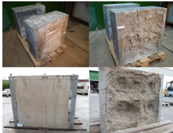
Figure 3. Specimen with 1 kg PP fibres per m 3 concrete after the experiment (left), specimen without PP fibres showing damage due to spalling (right).
