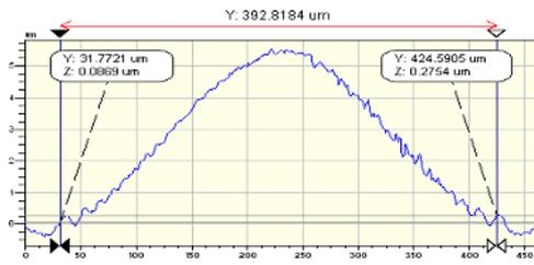
**Fig. 2.** Actual microbeam profile in microns at rest.
