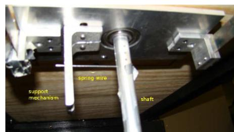
Fig. 2. Pitch spring mechanism.
