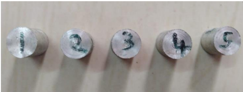
Fig. 5 Hardness test samples reinforced composites
