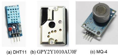
Fig. 3. Three sensors used in the experiment.
