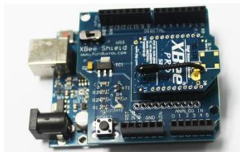
**Fig. 2.** Arduino, XBee shield and XBee Pro.
