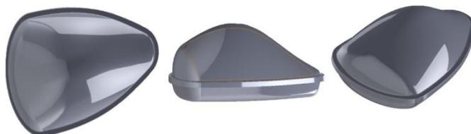
**Fig. 2.** Streamline roof box 3D model developed using CATIA V5.
