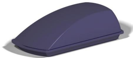
**Fig. 1.** Common roof box 3D model developed using CATIA V5.
