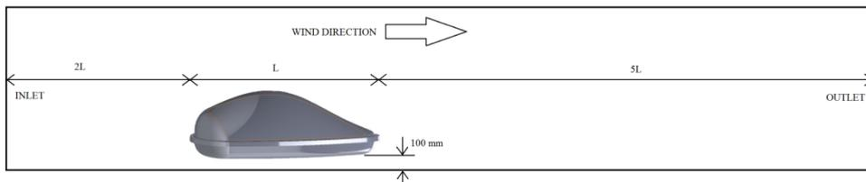
**Fig. 3.** MIRA Wind tunnel configuration.
