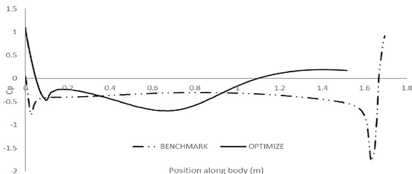
**Fig. 5.** Cp along upper body of both roof box
