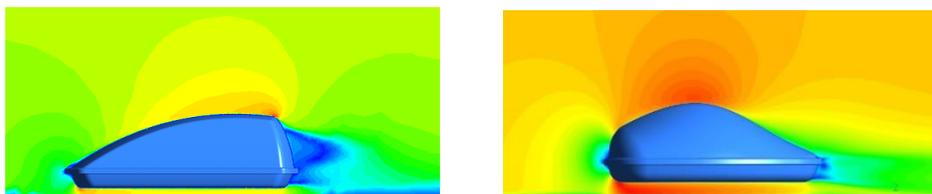
**Fig. 4.** Velocity contour of common and optimized roof box.
