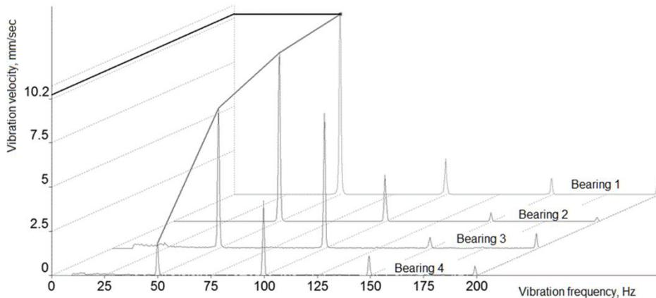
**Fig. 2.** Spectra cascade of vibration velocity, crosswise direction Maximal level (rate) – on bearing 1 (electric motor). Rotational frequency 50 Hz and amplitude 10.2 mm/sec. are designated by a cursor.
