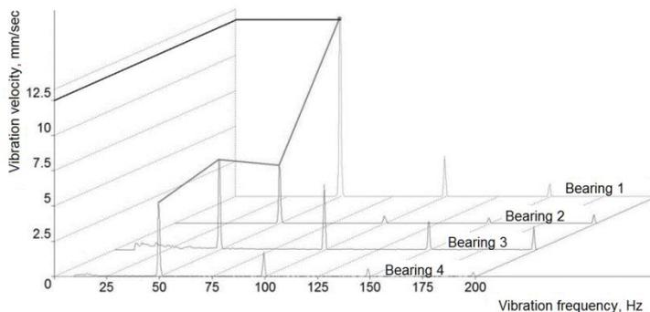
**Fig. 1.** Spectra cascade of vibration velocity, vertical direction.
