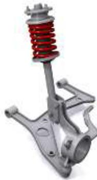
**Fig. 1.** MacPherson strut suspension.
