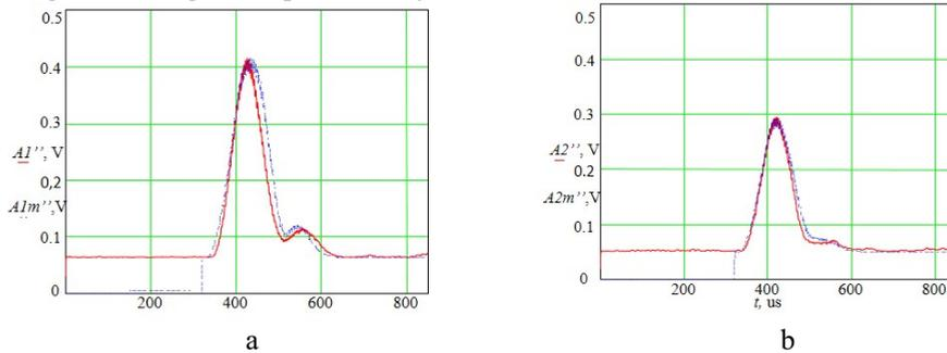
**Figure 5.** Envelope of the correlation of response 1 with the sounding signal and model signal envelope (a). Envelope of correlation of response 2 with the actuating signal and model signal envelope (b).
