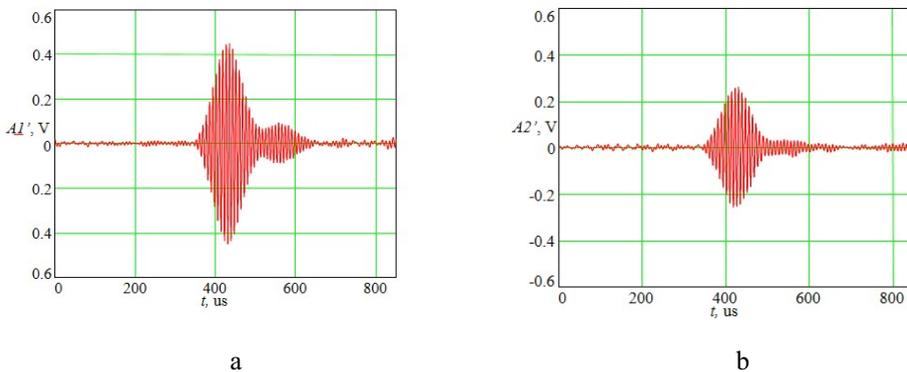
**Figure 4.** Correlation of response 1 from the defect-containing region and the acoustic signal (a). Correlation of response 1 from the defect-free region and the acoustic signal (b).
