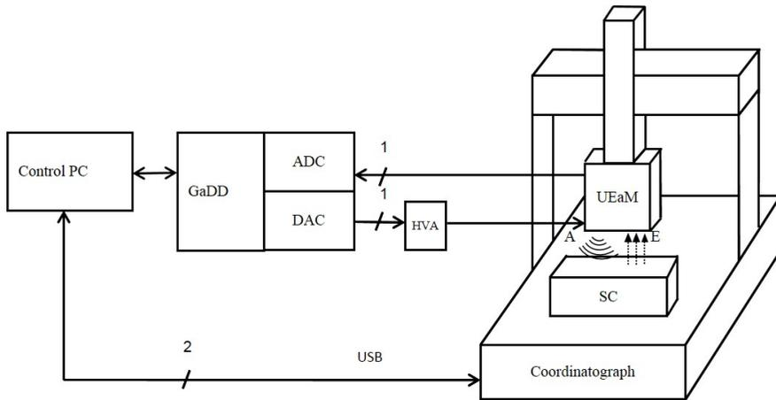
**Figure 1.** Block diagram of the experimental setup.
