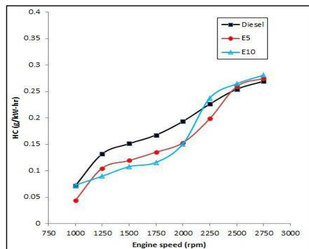
**Figure 8.** Hydrocarbon against engine speed
