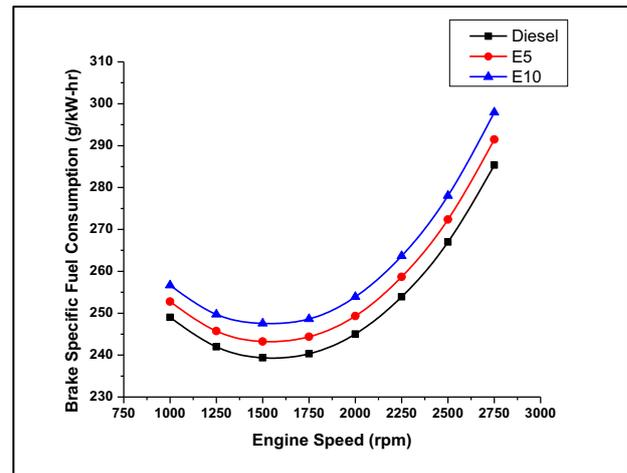
**Figure 7.** Brake specific fuel consumption against engine speed
