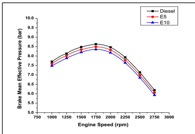
**Figure 6.** Brake mean effective pressure against engine speed
