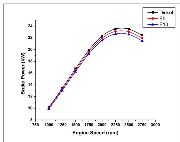
**Figure 5.** Brake power result against engine speed
