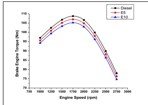
**Figure 4.** Brake engine torque against engine speed
