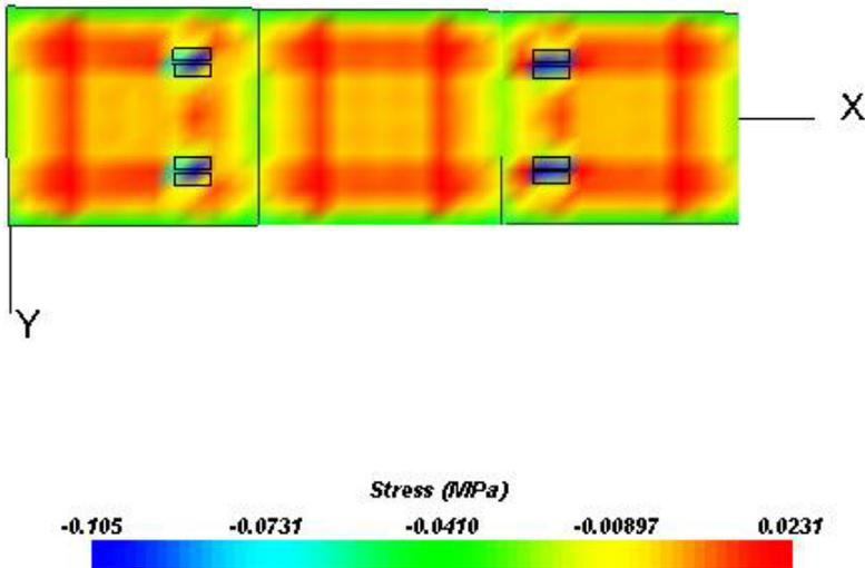
Fig 6. Stress in the z-z plane.
