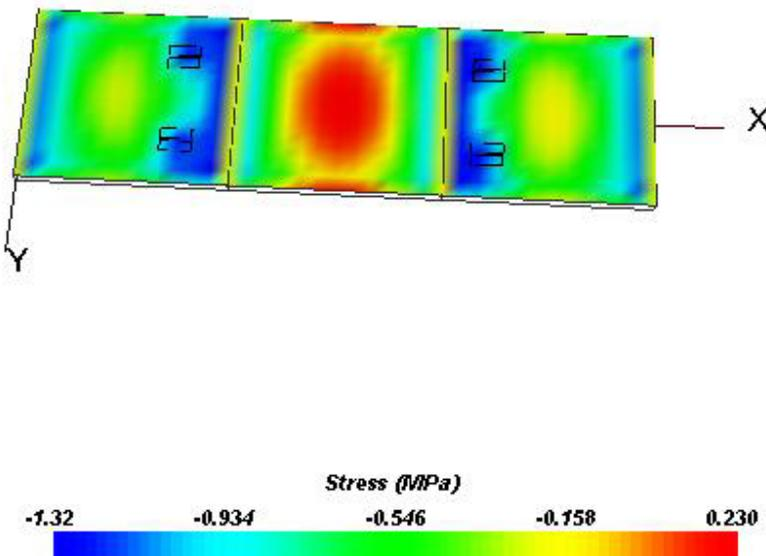
Fig. 5. Stress in the x-x plane.
