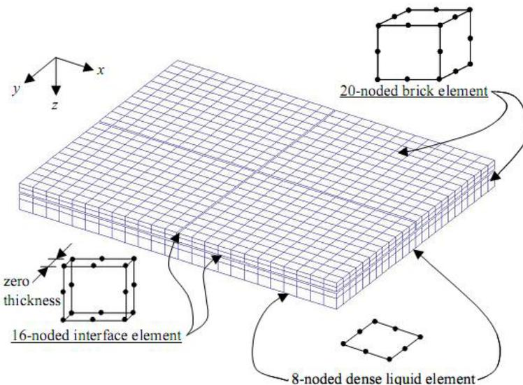
**Fig. 2.** The Basic Finite Element Discretization [2].
