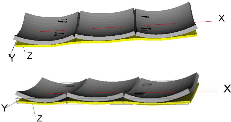
Fig. 7. Deflections of the all slabs and the base.
