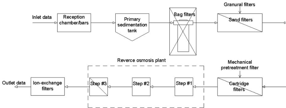
Fig. 3. Leachate Treatment Plant after Reconstruction.
