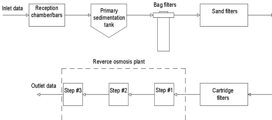
**Fig. 2.** Leachate Treatment Plant before Reconstruction.
