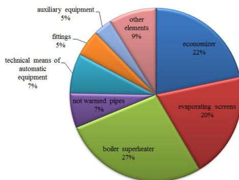
**Fig. 1.** The damaged elements of boiler aggregates.
