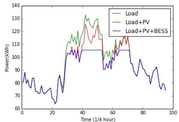
**Figure 4.** a) Load profile b) load profile with PV c) load profile with PV and BESS
