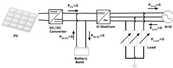
**Figure 3.** Microgrid structure with PV and BESS
