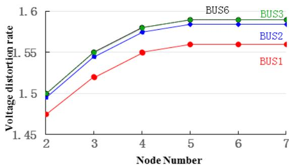
Figure 5. Total distortion rate under different access location.
