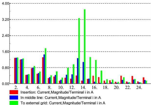
Figure 8. Harmonics in system without cable capacitance.
