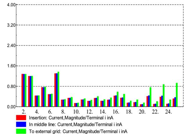
Figure 7. Harmonics in system without cable capacitance.
