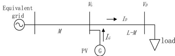
Figure 1. PV connected to distribution network.
