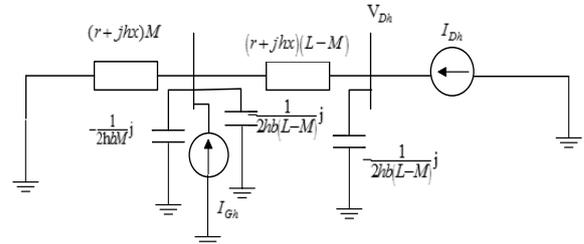
Figure 2. PV connected to distribution network model.
