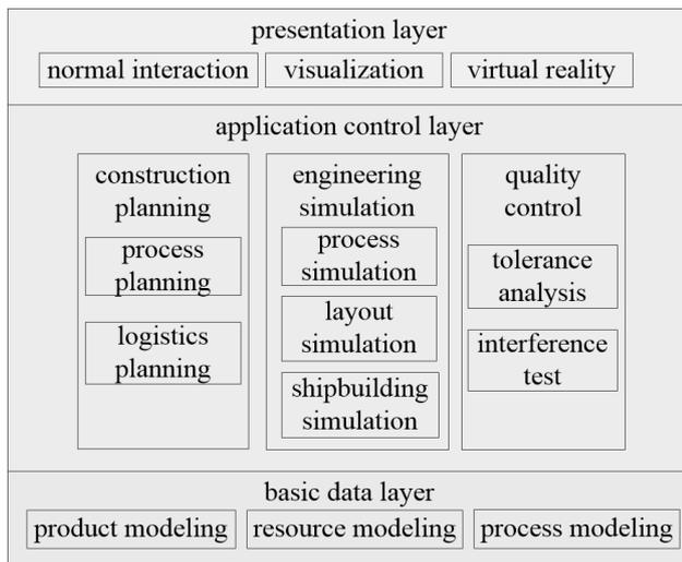
Figure 1. The digital factory hierarchy for shipbuilding
