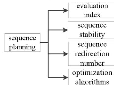
Figure 4. The constitution of sequence planning for shipbuilding
