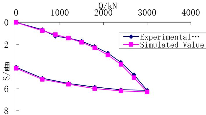
Fig.2 Comparison of Pile 2# top settlement relation with load.
