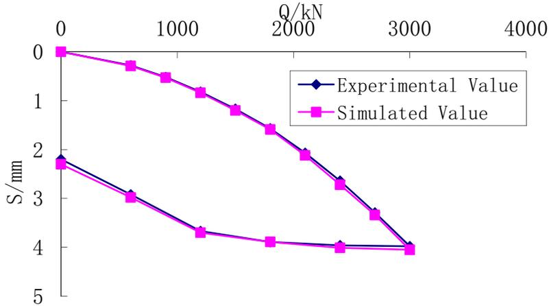
Fig.1 Comparison of Pile 1# top settlement relation with load.
