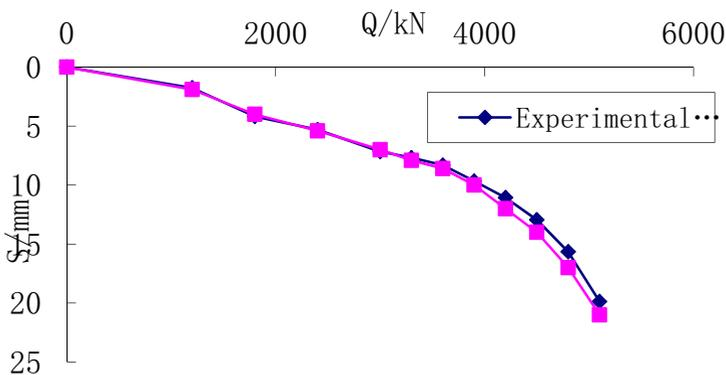
Fig.3 Comparison of Pile 3# top settlement relation with load.
