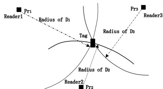
Figure 3-3 the signal strength of the positioning
