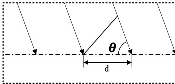
Figure 3-4 the received signal to determine the angle of arrival
