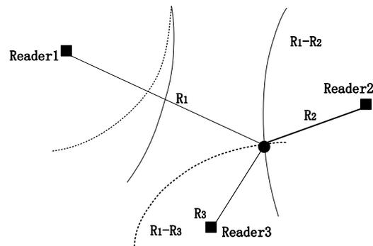
Figure 3-2 TDOA hyperbolic positioning method
