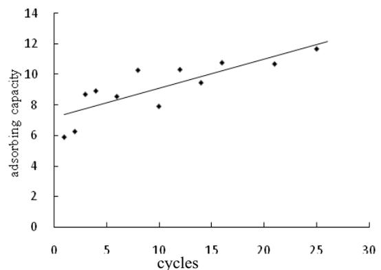
**Figure 5.** Adsorption capacity of biochar along 25 freeze-thaw cycles
