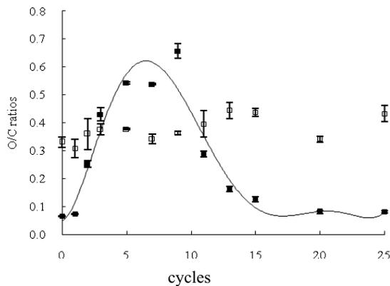
**Figure 2.** O/C ratios of biochar along 25 freeze-thaw cycles
