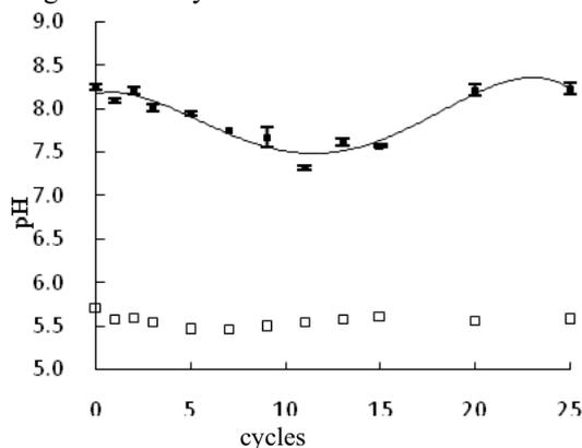
**Figure 3.** pH of husk biochar in 25cycles,
