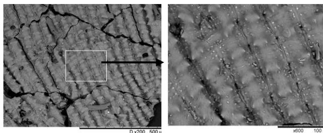
Figure 1. SEM of inside surface of husk biochar
