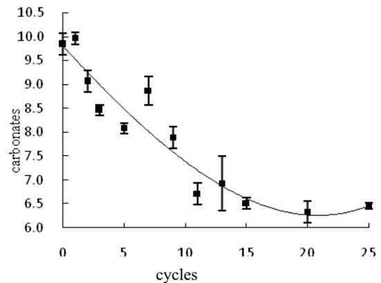
**Figure 4.** Carbonates content of biochar along 25 freeze-thaw cycles
