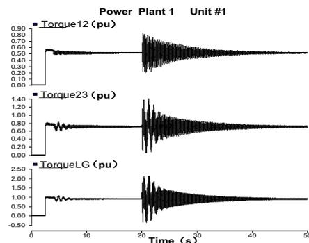
**Figure 3.** Power plant 1 -unit #1 torque change between each mass when having the 750kV equivalent source
