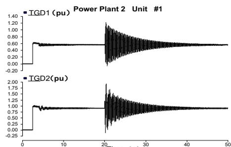
**Figure 5.** Power plant 2 -unit #1 torque change between each mass when having the 750kV equivalent source
