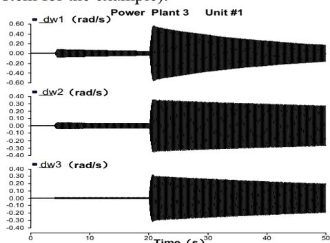
**Figure 6.** Power plant 3 -unit #1 each modal shaft speed deviation when having the 750kV equivalent source
