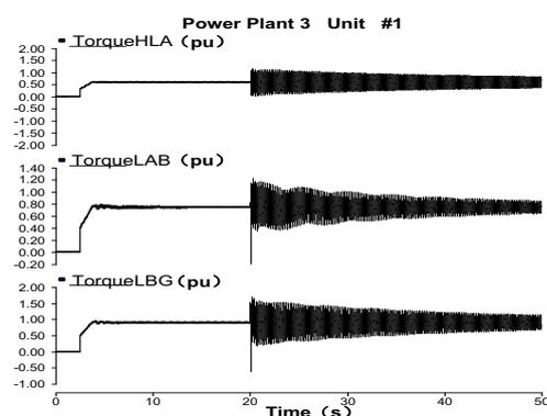
**Figure 9.** Power plant 3-unit #1 torque change between each mass at which not having the 750kV equivalent source
