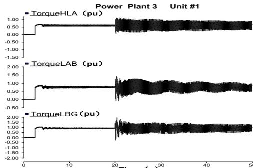
**Figure 7.** Power plant 3 -unit #1 torque change between each mass when having the 750kV equivalent source
