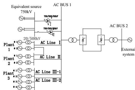
**Figure 1.** The Researched UHVDC Equivalent Network Diagram
