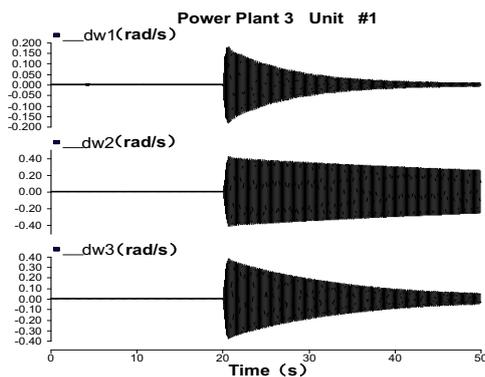
**Figure 8.** Power plant 3-unit #1 each modal shaft speed deviation at which not having the 750kV equivalent source
