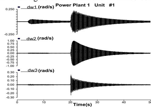
**Figure 2.** Power plant 1 -unit #1 each modal shaft speed deviation when having the 750kV equivalent source
