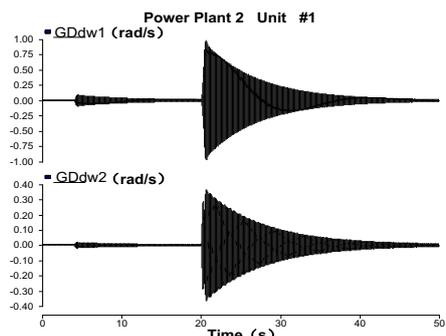
**Figure 4.** Power plant 2 -unit #1 each modal shaft speed deviation when having the 750kV equivalent source
