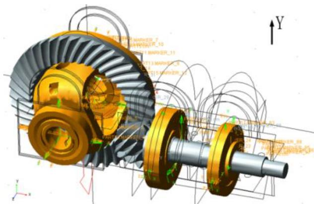
**Figure 5.**Dynamic model of the main reducer gear system
