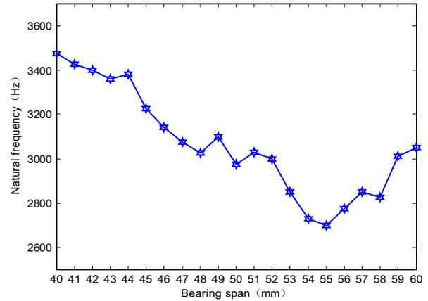
Figure 3. Natural frequencies - bearing span
