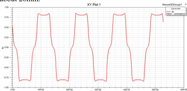
(a) air gap center line magnetic density curve corresponding to the figure3 (a)
