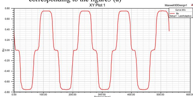
(b) air gap center line magnetic density curve corresponding to the figure3 (b)
