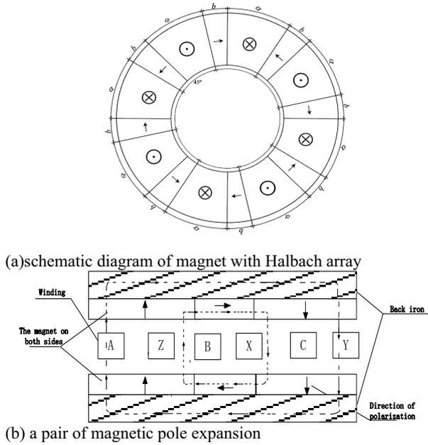
**Figure 1.** the expand structure of disc type generator with 90° Halbach array
