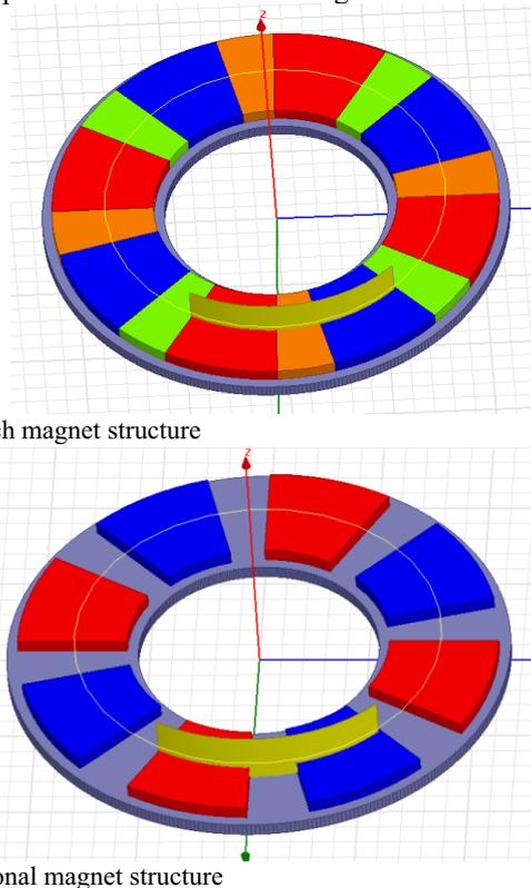
**Figure 3.** finite element model of disk type generator
