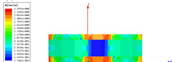
(b) the magnetic flux density corresponding to the section in figure3(b)
