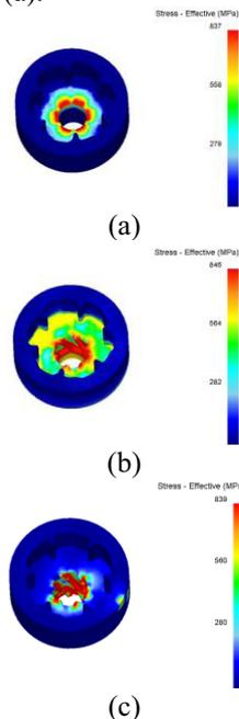
**Figure.7** Billet equivalent stress distribution of the rotary forging: (a) the initial forming stage, (b) the middle forming stage, (c) the final forming stage.
