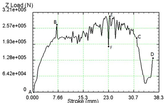
**Figure. 5** The forming load result of the rotary forging process.
