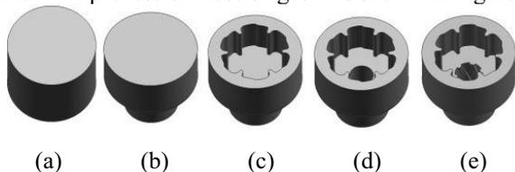
**Figure. 2** The forming process of automotive guide cylinder: (a) making billet, (b) forward extrusion, and upsetting, (c) backward extrusion cavity, (d)making guiding hole,(e) cold rotary forging internal helical involute spline.
