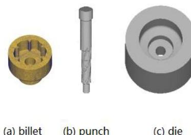
**Figure. 4** Finite element model: (a) billet, (b) punch, (c) die.
