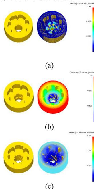
**Figure.6** Billet deformation and metal flow results of rotary forging: (a) the initial forming stage, (b) the middle forming stage,(c) the final forming stage.
