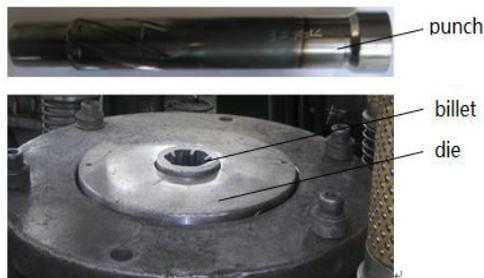
Figure. 8 Tools used for the experiment.
