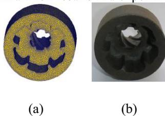
Figure. 9 Models comparison: (a) the simulated model, (b) the experimental model.
