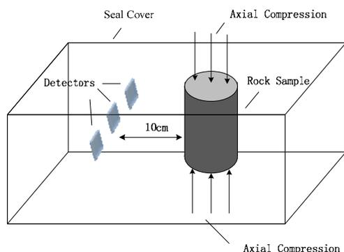
**Fig.1** Schematic sketch of Radon measurement device
