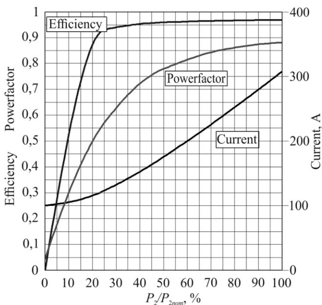
**Figure 1.** Characteristics of the 500 kW MORLEY motor
