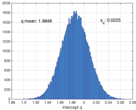
**Figure 4.** Calibration line relative to the Young modulus (on the top) with  $N=100\ 000$  determined by means the Monte Carlo method. The lines relative to  $m \pm s_m$  and  $q \pm s_q$  have been added in the plot. The pseudo-Gaussian distribution of the  $m$  and  $q$  coefficients (on the bottom).
