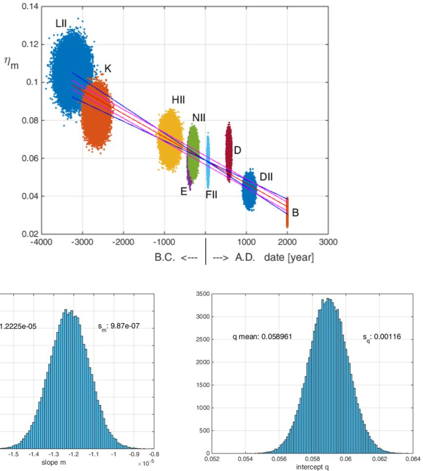
**Figure 5.** Calibration line relative to the loss factor (on the top) with  $N=100\ 000$  determined by means the Monte Carlo method. The lines relative to  $m \pm s_m$  and  $q \pm s_q$  have been added in the plot. The pseudo-Gaussian distribution of the  $m$  and  $q$  coefficients (on the bottom).
