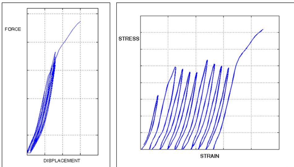
**Figure 1.** Example of the result of a cyclic loading test on a fiber (on the left), and the same result (on the right) obtained after a proper processing addressed to highlight the sequence of cycles.
