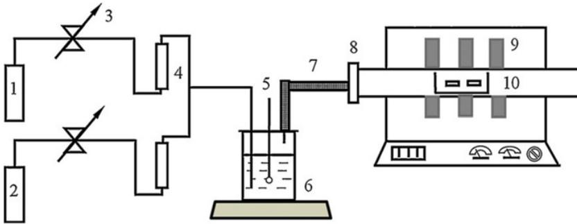
**Figure 1.** Schematic diagram of the oxidation experiment set. (1) Oxygen, (2) nitrogen, (3) valve, (4) flow meter, (5) thermometer, (6) water bath, (7) heater band, (8) seal ring, (9) heating unit and (10) specimens.
