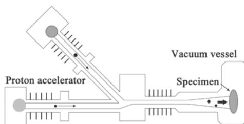
**Figure 4.** Ground based space radiation environment simulator.
