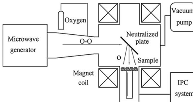
**Figure 2.** Coaxial source atomic oxygen ground-based simulation facility.
