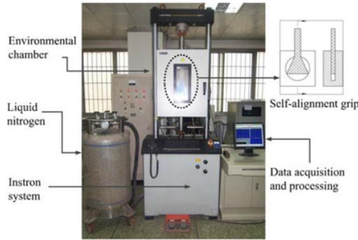
**Figure 3.** The cryogenic experimental system.
