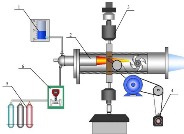
**Figure 5.** The schematic diagram of the experimental simulation method. 1, water-cooling system; 2, atmospheric subsonic gas-fired wind tunnel; 3, loading system for mechanical property tests; 4, servo-actuator of the rotating system; 5, gas supply; 6, mass flow controller of gas.
