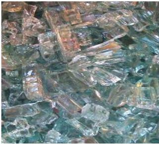
**Figure 1.** Crushed waste glass that used as an additional material in concrete
