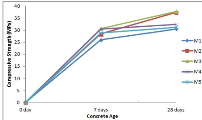
**Figure 2.** The compressive strength of special concrete
