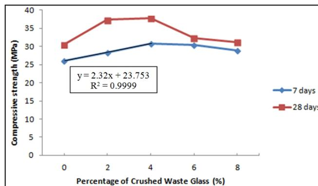
**Figure 3.** The relationship between the compressive strength with percentage of crushed waste glass.
