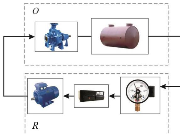
**Figure 2.** System two-position control level in the tank.
