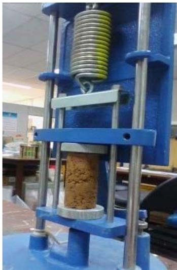
Figure 5. Placement of specimen
