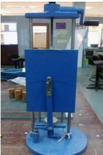
Figure 4. Apparatus for UCS test
