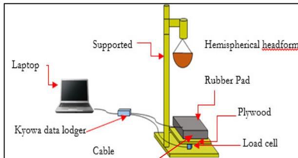
**Fig. 2:** Apparatus drop test set up
