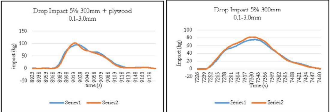
Fig. 4: Example graph of drop impact
