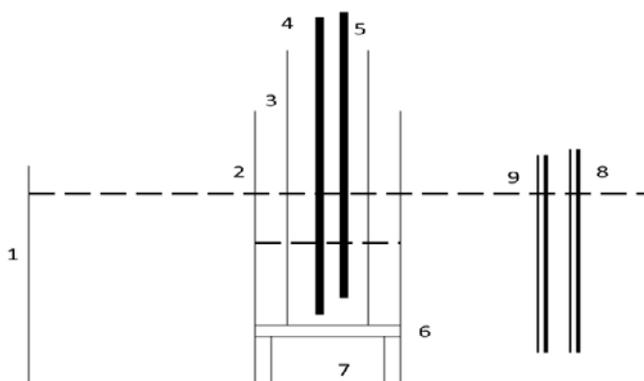
**Figure 1.** Wax deposition setup. (1) Cold bath, (2) pipe, (3) mould, (4) heating rod connected temperature controller, (5) thermocouple, (6) rubber gasket, (7) supporter, (8) cooling water inlet, (9) cooling water outlet.
