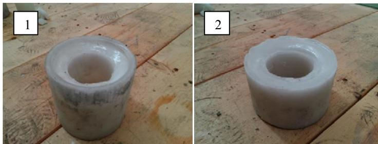
**Figure 2.** (1) Wax deposit using new system, (2) wax deposit using pour casting method.
